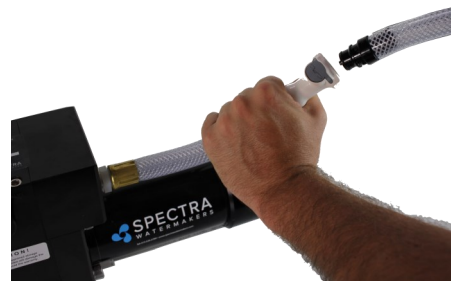
Attaching brine discharge service hose 49
