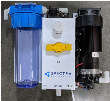
Service valve OFF
