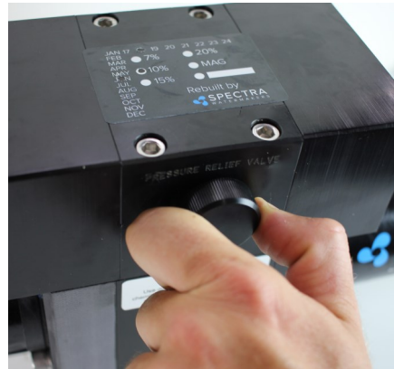
Open 1/2 Turn when purging chemicals!
