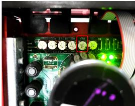
3. You will be adjusting the potentiometer that can be found second from the far right. The potentiometer will read "MAX" labeled upside down. Turn the screwdriver left to slow the Boost Pump speed and reduce the Boost Pressure or turn the screwdriver right to increase Boost Pump Speed.
