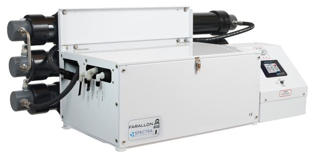
The membrane maximum temperature specification is 113°F (45°C), as specified by the membrane manufacturer. This module must be installed in an area that maintains a temperature below 120F (50C). Make sure that the area around and under the pump does not have any water sensitive equipment. Water will be spilled during any repairs or if a leak occurs.
