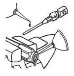
4. Oil nipple threads and inside of hose with silicone oil or diluted soapy water. DO NOT OIL HOSE COVER
