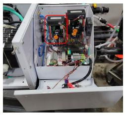
2. You will need a small Phillips head screwdriver to adjust one of the potentiometers on the left VFD (Variable Frequency Drive).
