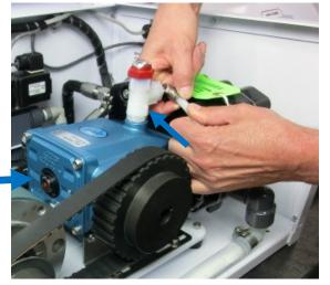
Drain oil into a suitable container.
