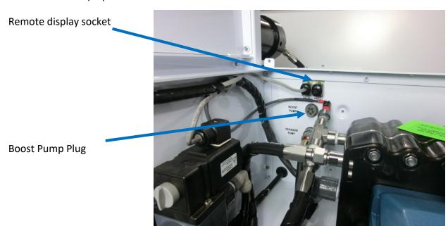
Route the boost pump power cable to the Control Box from the boost pump. Do not get the cable wet, and be careful not to damage the plug or conductors during installation. The boost pump power cable plug is located under the sockets for the Salinity probe and the Remote display. Route the power cable and use cable ties to keep it in place.
