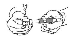
2. When assembling male pipe ends, slide nipple onto mandrel.
