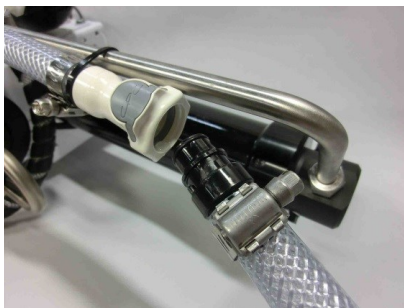
Connecting brine discharge service hose
