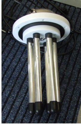
Anodes fitted on to the header without cathodes
