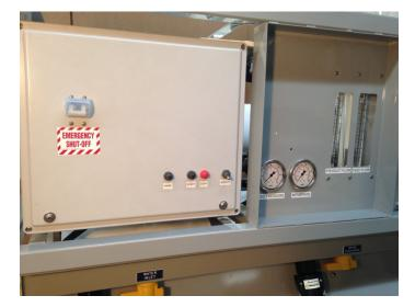
The service switch will run the Pearson Pump only (no feed pump) on service speed (about 1/2 speed or 10 gpm) for fresh water flushing, cleaning or pickling.
