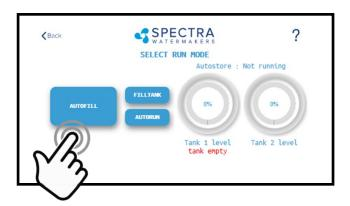
In Auto Fill Mode the Spectra Connect will automatically fill your water tank, stop itself, fresh water flush, return to Auto Store mode with the flush interval timer running, and then turn itself on again to fill the tank as soon as the water level drops below the Tank Low Switch with no additional user commands.
