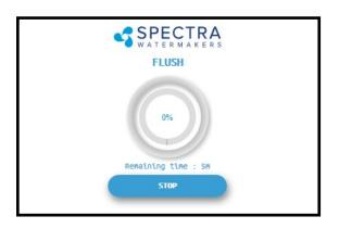
Note: If the pump is knocking during the flush cycle changing the pump speed (either up or down) can help. This is done in the Dealer Access section by changing the "Pump 3" settings. Pump 3 are the voltage settings for the different run speeds, 10 volts is full speed, 5 volts is half speed. The system needs to be stopped to make this adjustment and you need to save the setting before restarting.
