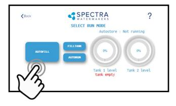
In Auto Fill Mode the Spectra Connect will automatically fill your water tank, stop itself, fresh water flush, return to Auto Store mode with the flush interval timer running, and then turn itself on again to fill the tank as soon as the water level drops below the Tank Low Switch with no additional user commands.
