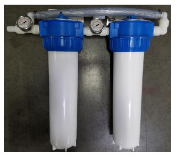
*Note:* Filter housings should always be tightened by hand, do not use the wrench. Overtightening the collar will not improve sealing. If the housing leaks when hand tightened then the O-ring needs to be cleaned and greased (silicone grease only). A small amount of silicone grease on the threads will make it easier to remove the collar.
