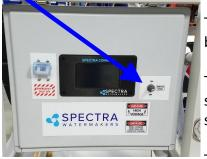
Turn the Service switch to off, remove the brine hose from the bucket and put it to a drain.
