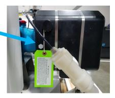
**Technical tip:** Knocking in the Pearson Pump is caused by the boost pressure being either too low or too high. Adjust the boost pressure as high as possible and close the brine discharge valve to add 3-5psi of back pressure.
