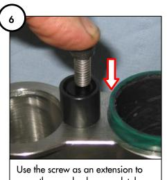
press the spool valve completely into the borehole.
