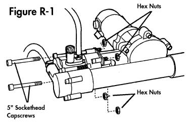
shaft (see Figure 8). Be aware that the coupling pin fits loosely in the drive shaft and may fall out when the rubber boot is removed. Be careful not to lose it. Separate the drive assembly from the pump and set the drive assembly aside.
