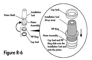
**Note:** This is a very tight fit by design and will require a fair amount of force to push the PIP ring down the installation tool. You may use an object to help push the pip ring evenly down the tool. Please make sure not to damage the PIP ring.
