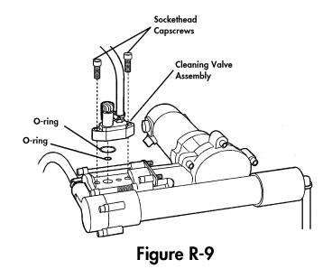
cleaning valve assembly on the pump body and install the two cap screws. This completes the procedure for reassembly of the watermaker. When operation is commenced again, carefully inspect the watermaker for proper operation and any leaks or other signs of incorrect assembly.
