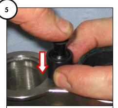
Press the spool valve by hand into the borehole.
