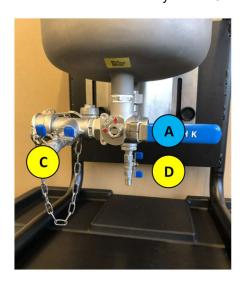
After being prepared based on DIN EN 2557-2, the water sample can be taken by opening the sampling valve D.
