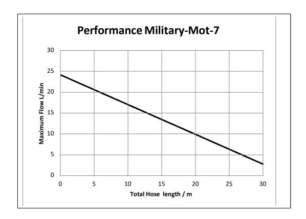
The above chart shows the typical performance of the unit when operated in the standard operating conditions described in this manual. Increasing the static resistance of the system through the use of a longer supply and connection hoses will reduce the volume of purified water. Optimal positioning of the intake hose (reducing dirt intake) and reducing the hose lengths increases the performance of the MOT-7.
