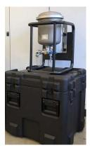
• Remove the filter unit from its storage carton and position it at the appropriately comfortable height for operation and maintenance. Take care that the filter unit is placed in a stable position and that the location surface is dry.
