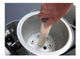
Remove the No. 5 filter elements from the storage area and screw them hand-tight into the filter housing. Pay particular attention that that you do not tighten them too much. Over tightening can damage the filters
