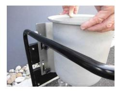
Loosen the locking mechanism and lift the filter holder to place it in the higher of the working positions. Then pull the locking mechanism closed again.
