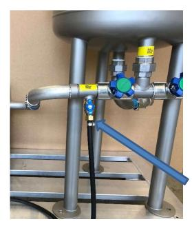
Hook up the cleaning hose to the corresponding threads. The MOT-31/54 is now ready for use.
