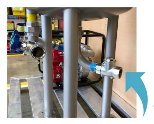
After being prepared based on DIN EN 2557-2, the water sample must be taken at the outlet of the filter
