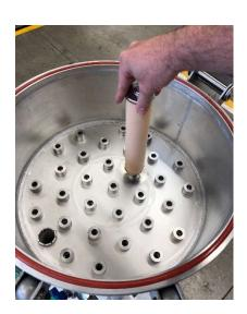
Remove the No. 5 filter elements from the package and screw them hand-tight into the filter housing. Pay particular attention that you do not tighten them too much. Over tightening can damage the filters.
