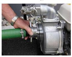
Connect the suction hose for untreated water to the pump and position the intake filter in the water at the intended site based on the description in the operating instructions.
